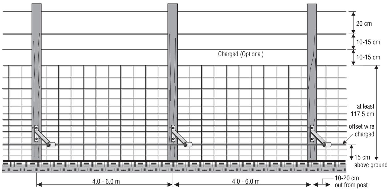
Figure 2. An electrified, high tensile mesh-wire fence, viewed from outside the enclosure
