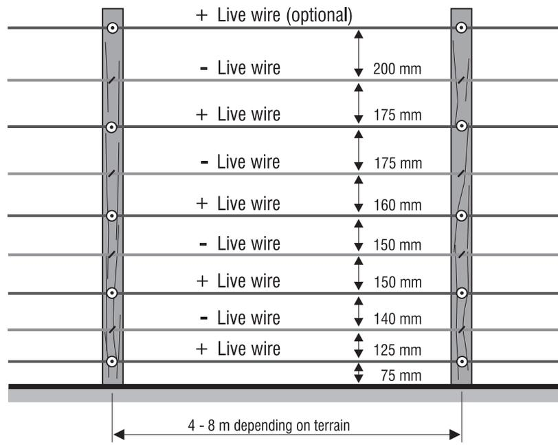
Figure 1. Nine-wire electric fence, viewed from the inside the fence
